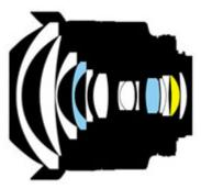
Aspherical lens elementsED glass elements E: Super ED glass elements
